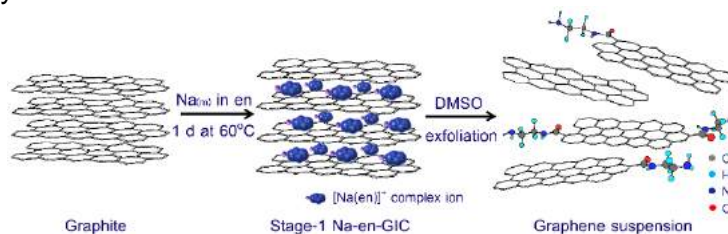
Fig. 1 Synthesis route of the graphene suspension from a stage-1 GIC.
