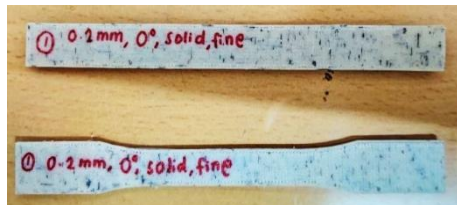
Fig. 1: Printed specimens ABS- oil palm fiber composite (3wt%)
