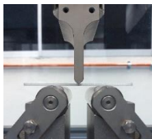
Fig. 2: Setting of specimens with 50mm gauge length
