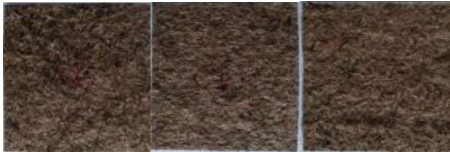
Fig 1: Fiber weight percentage in composite 30 wt.% 40 wt.% 50 wt.%
