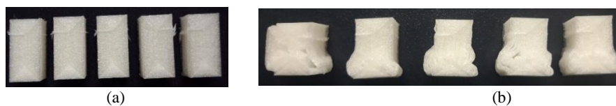
Fig. 2: Compression Specimen (a) before the test (b) after the test
