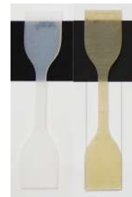
Figure 2: The UHMWPE/CNF nanocomposite and neat UHMWPE
