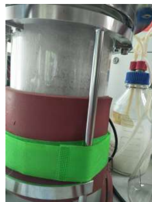
Figure 1: Fermentation of biosurfactant in 2L bioreactor.
