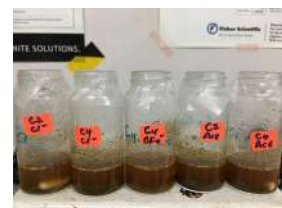
Figure 2: Extraction of phenolic acids from lemongrass leaves using ionic liquids.
