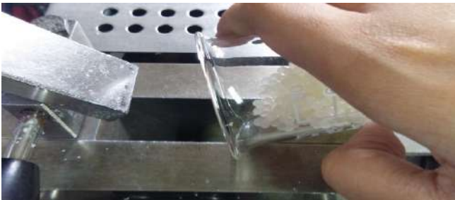
Figure 1: Preparation of PLA/CNF nanocomposite using internal mixer (Brabender)
