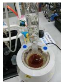
Figure 2: Mixture of oil, sulphuric acid and methanol was refluxed for 3 hours.
