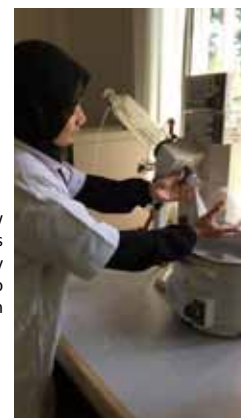
Figure 3. Raw biosurfactant was dried using a rotary evaporator prior to purification
