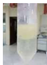
Figure 2. Biosurfactant precipitates in acidic condition
