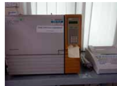
Figure 2. Determination of ABE and organic acids using gas chromatography (Model GC-17A, Shimadzu, Japan)
