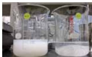
Figure 1. Purification of dissolved PHB powder in methanol and hexane.
