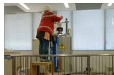
Figure 4. Placing the sample's tube in the 500-MHz JEOL JNM-ECP500 FT NMR system.
