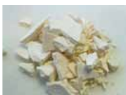
Figure 1. Polyester from lipase-catalyzed of dicarboxylic acids and diols
