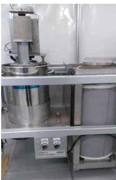
Figure 1. Sand bath reactor for hydrothermal process
