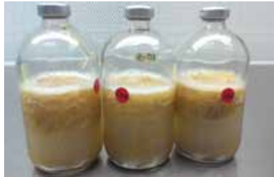
Figure 1. Fermentation of simultaneous saccharification and fermentation for biobutanol production
