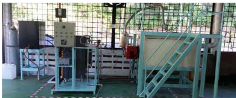
Figure 1. Carbonisation-activation system for the production of biochar and activated carbon.
