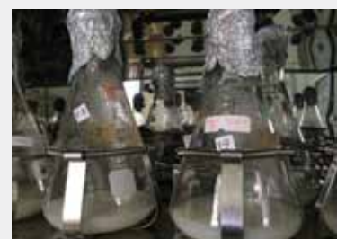
Figure 1. Production of biosurfactant in incubator shaker by local isolate
