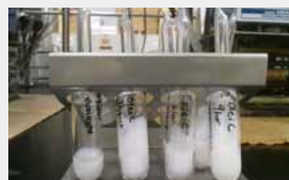
Figure 1. Polyester from lipase-catalyzed of dicarboxylic acids and diols
