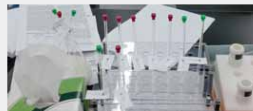
Figure 3. Prepared hydrolyzate samples in NMR tubes for proton NMR analysis
