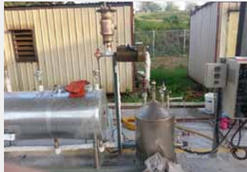
Figure 1. Reactor used for carbonization and activation
