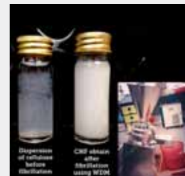
Figure 3. Fibrillation using wet disc milling (WDM)
