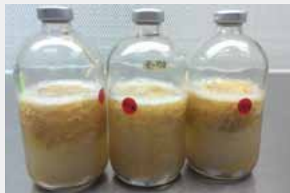
Figure 1. Fermentation of simultaneous saccharification and fermentation for biobutanol production
