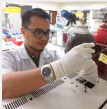
Figure 1. Sample injection into Gas Chromatography bioreactor
