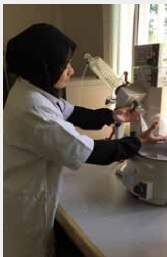
Figure 2. Raw biosurfactant was dried using a rotavap prior to purification
