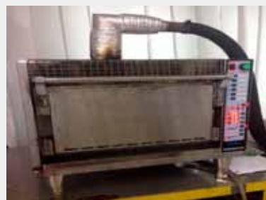
Figure 1. Superheated steam pretreatment of OPMF and OPEFB
