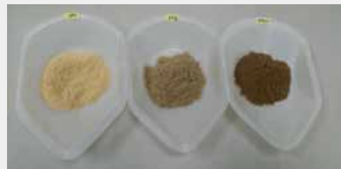
Figure 1. Oil palm biomass involved in pretreatment that are frond (OPF), empty fruit bunch (OPEFB), and mesocarp fibre (OPMF).
