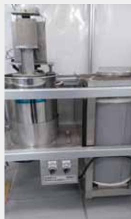
Figure 1. Sand bath reactor for hydrothermal process
