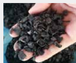
Figure 2. Activated carbon of palm kernel shell obtained using two-in-one carbonisation and activation system.
