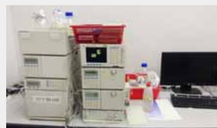
Figure 2. HPLC used for organic acid analysis
