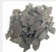
Figure 1. Biochar from coconut shell used as treatment to improve composting process
