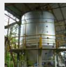
Figure 2. Composting bioreactor of 10 m 3 size
