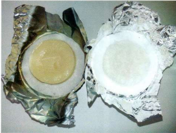
Differences between untreated (left) and hydrothermal pretreated (right) samples during lignocellulosic compound determination.
