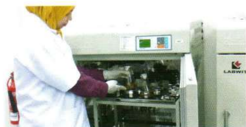
Figure 3: Substrate pretreatment using cellulase enzyme prior to hydrodistillation
