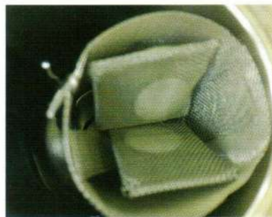
PHB disks arrangement prior to steam hydrolysis
