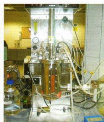
Bioethanol fermentation using hydrolysate of sago hampas in 3L bioreactor.
