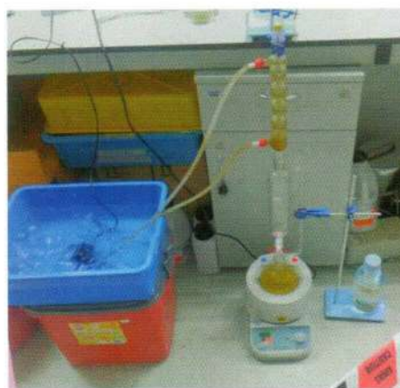
Figure 2: The hydrodistillation set up
