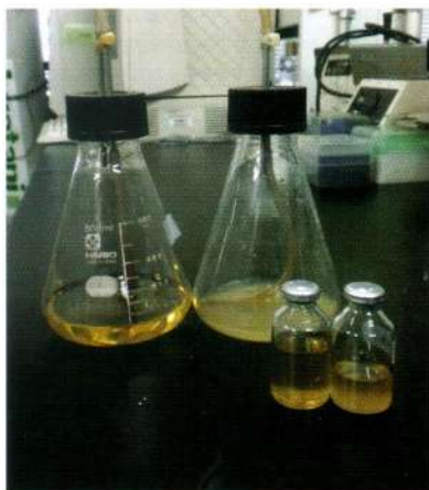
Small serum bottles and anaerobic flask were used for fermentation purposes.
