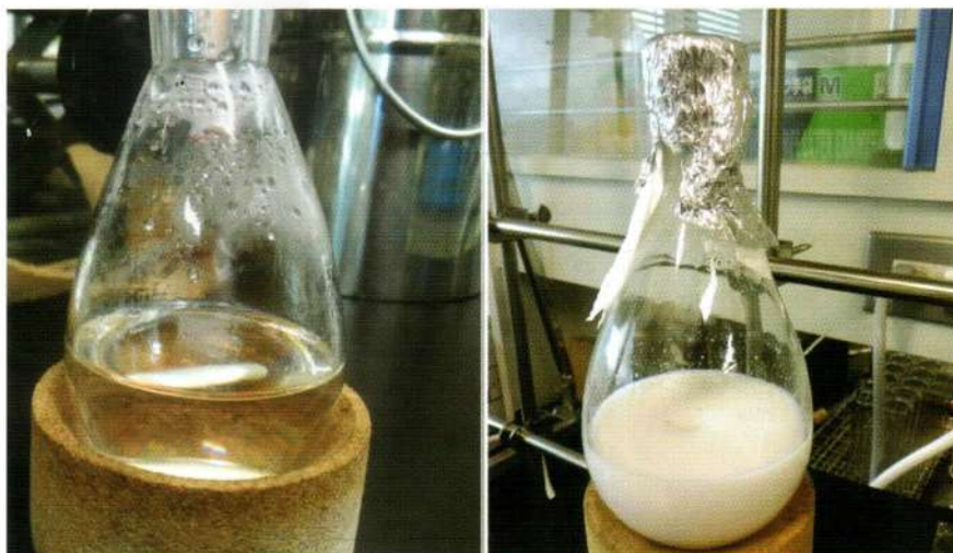
Synthesis of dicarboxylic acid monomers from metathesis of oleic acid by 2nd generation Grubbs catalyst.
