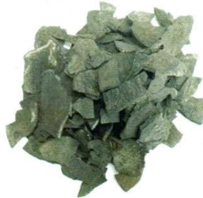
Biochar from coconut shell used as treatment to improve composting process
