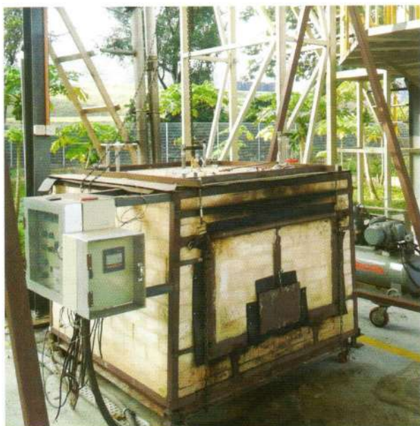
Fig.1 Pilot Scale (30 kg) brick self-sustained carbonization reactor
