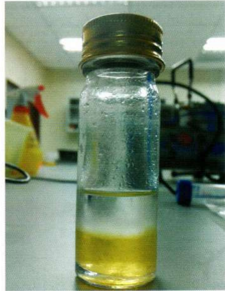
Fatty acids methyl esters of used cooking oil, FAME (upper layer) and hexane (lower layer)
