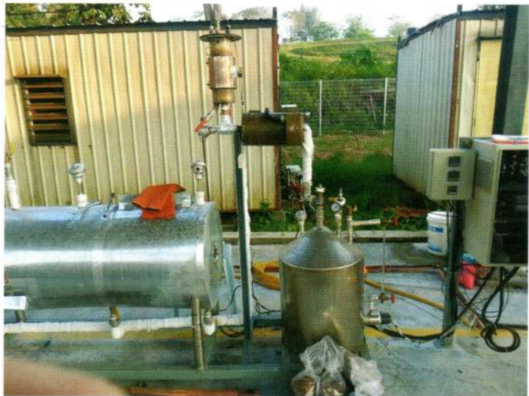
Reactor used for carbonization and activation
