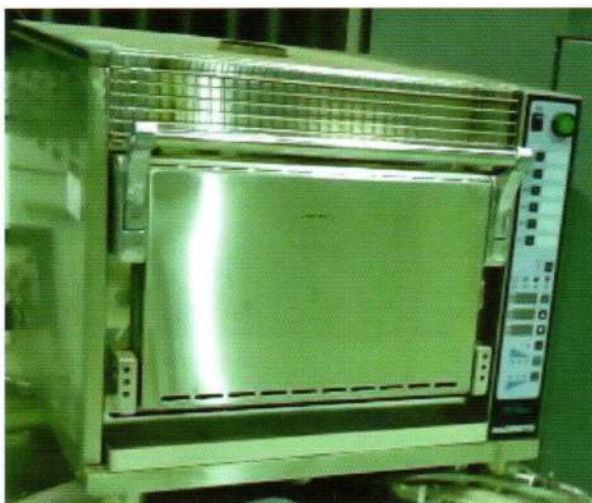
Figure 2: Superheated steam (SHS) oven used for depolymerization of PHA
