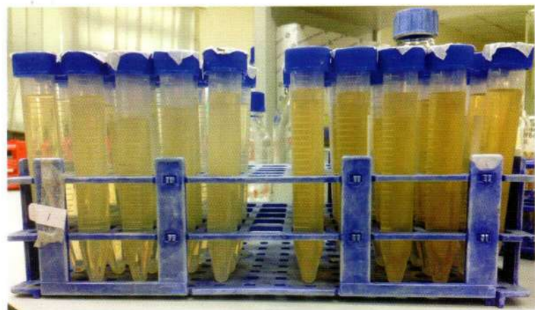
Untreated OPEFB and SHS pretreated OPEFB after saccharification
