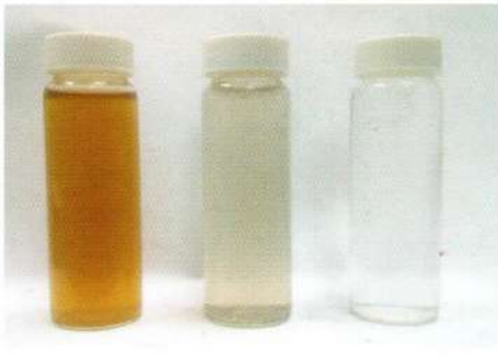
Palm oil mill final discharge before (left) and after treatment (right) with mesocarp fiber activated carbon. Tap water for comparison (right)
