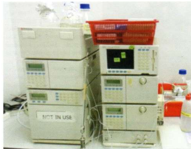
Figure 3 : HPLC used for organic acid analysis
