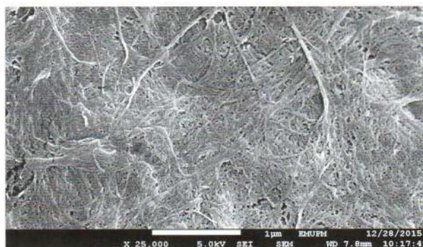
Nanofiber produced by wet disk milling
