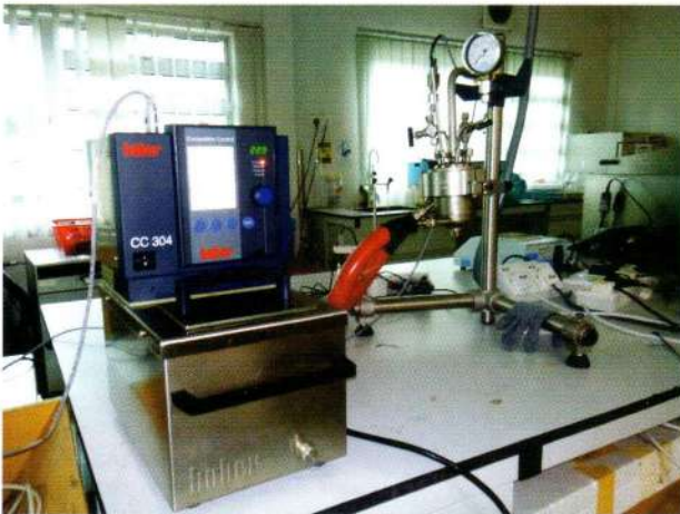
Machine used for steam explosion pretreatment (Huber CC-304B Thermostat).
