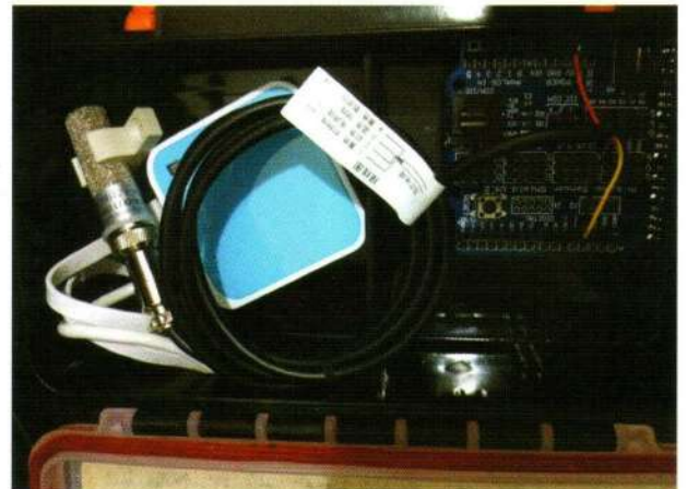
Temperature and Humidity Sensor with Datalogger
