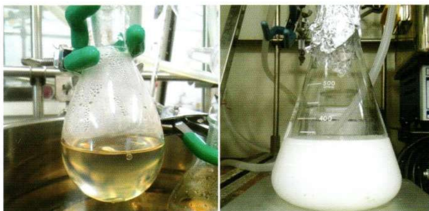
Synthesis of polyester from dicarboxylic acid monomers with aliphatic / aromatic diols by using isopropyl titanate.
