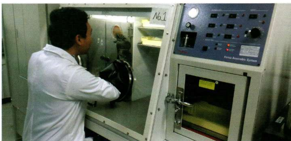
Inoculum was transferred into vials containing media in an anaerobic chamber.
