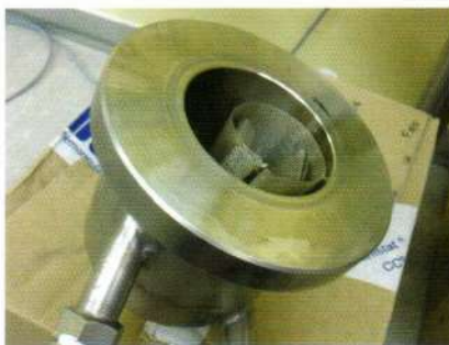
Saturated steam reactor: bottom part
