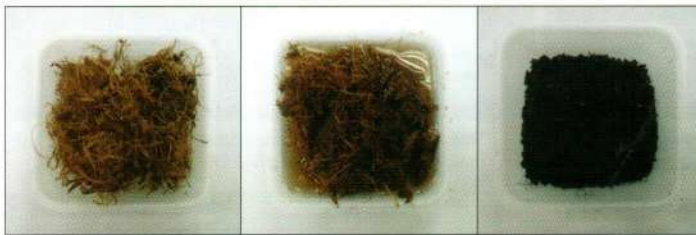
From left: Raw mesocarp fiber, mesocarp fiber during impregnation, activated mesocarp fiber
